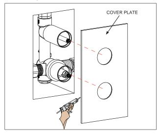
Apply a narrow bead of clear silicone sealant around the back edge of the cover plate and carefully press into position.
